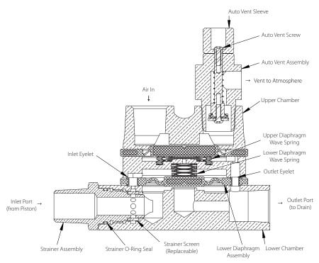
The Series 776 Low-Pressure Actuator is located on the trim of pneumatically released Victaulic dry, deluge, and preaction valves and comes standard on the Series 768 Dry, 769 Deluge, and 769 Preaction FireLock NXT Valves. The Series 776 acts as the trigger for these systems.
