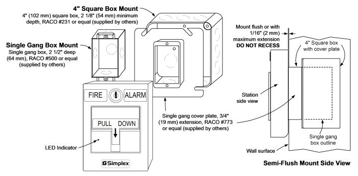
Figure 1: Addressable Manual Station Semi-Flush Mounting
