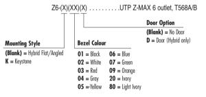
Outlet terminates UTP cable constructions with 23 – 26 AWG (0.64 – 0.51mm) solid and 26 AWG (0.48mm) stranded conductors, with up to 0.60mm diameter conductors and up to 1.48mm diameter over insulation.
